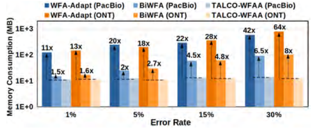
Fig. 12: Memory footprint of a single-thread CPU execution of WFA-Adapt, BiWFA, and TALCO-WFAA for 50Kbp PacBio and ONT reads at error rates.
